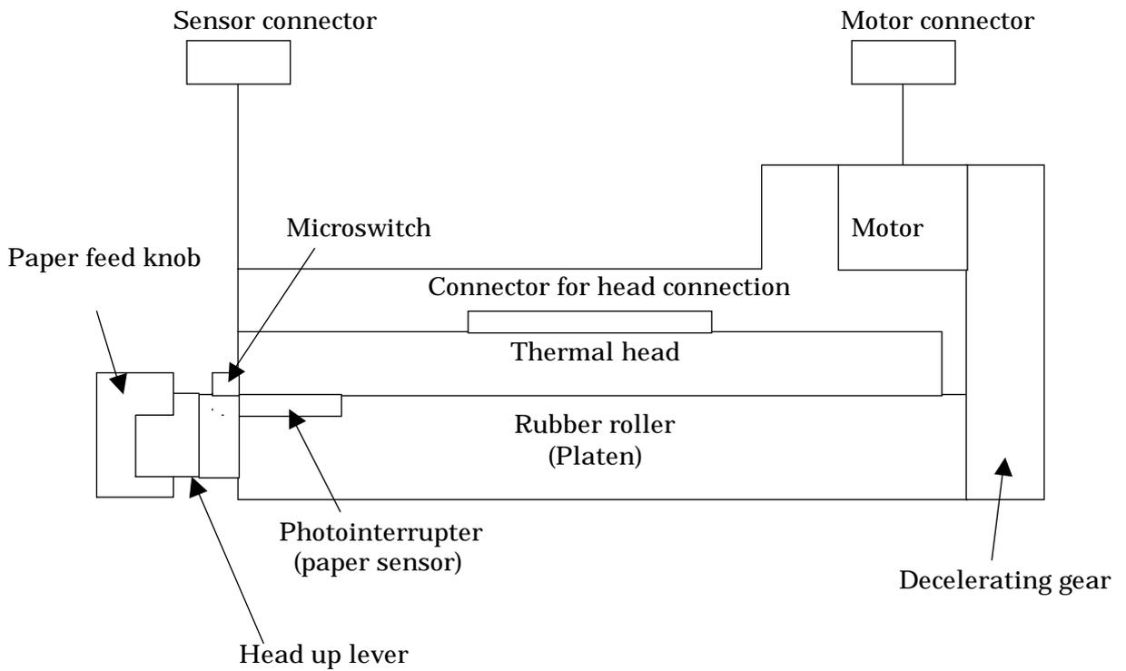
Figure 1 Printer configuration
