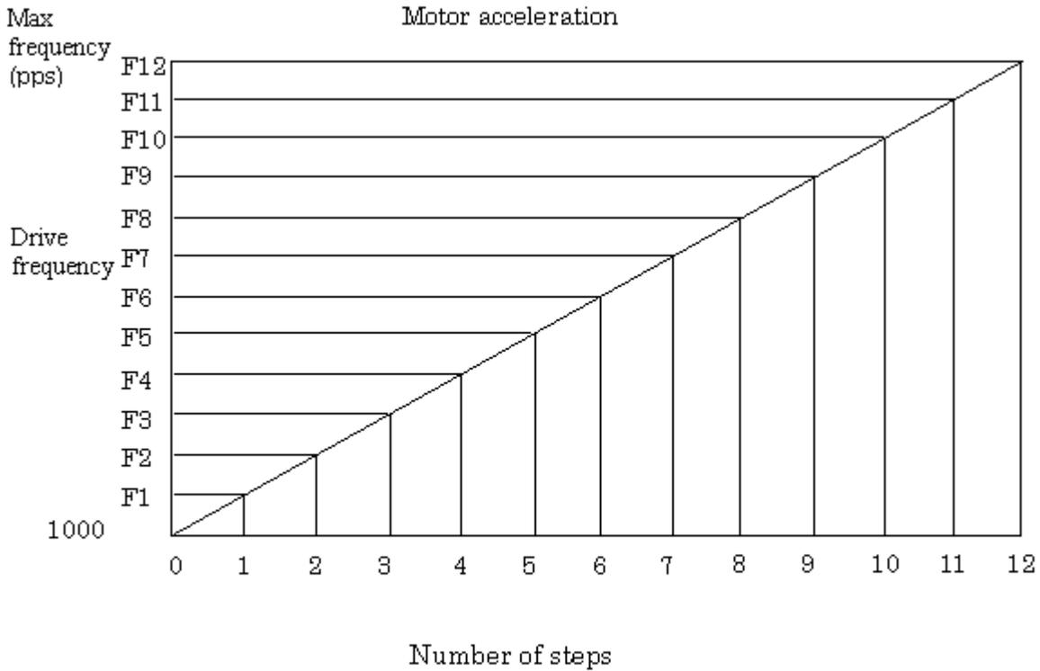
(b) If motor excitation is off when acceleration is started, feed current though the motor for about eight ms beforehand.
