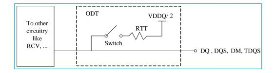
The switch is enabled by the internal ODT control logic, which uses the external ODT pin and other control information. The value of RTT is determined by the settings of Mode Register bits. The ODT pin will be ignored if the Mode Register MR1 and MR2 are programmed to disable ODT and in self-refresh mode.
