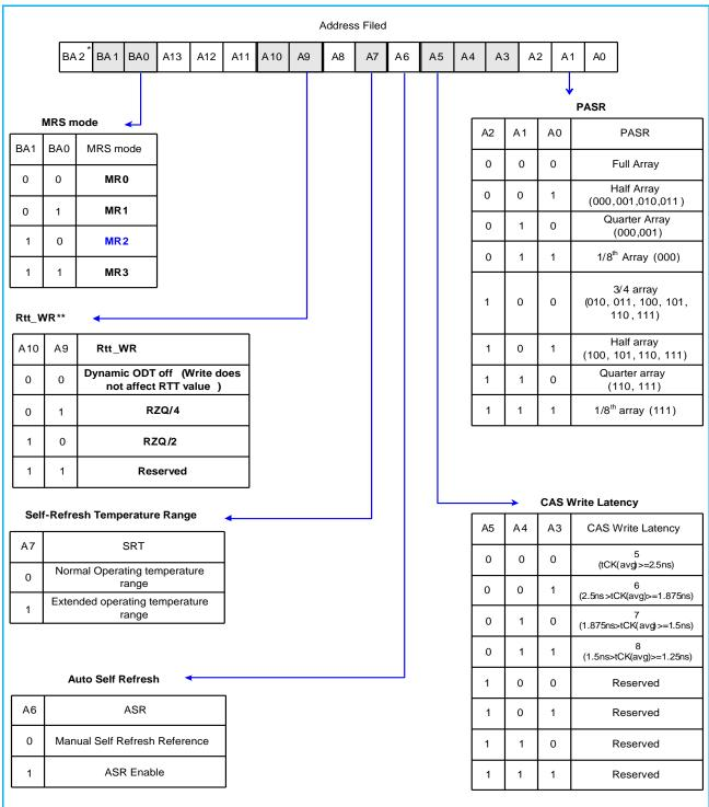
\* BA2, A5, A8, A13 are reserved for future use and must be set to 0 when programming the MR \*\* The Rtt\_WR value can be applied during writes even when Rtt \_\_Nom is disabled . During write leveling , Dynamic ODT is not available
